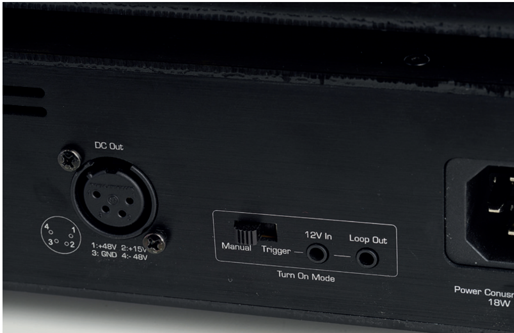
The Spower provides an unsymmetrical voltage of 15 volts and a symmetrical voltage of plus/minus 48 volts. It can be put into operation from standby mode via the switch on the front panel or a trigger voltage of 12 volts
