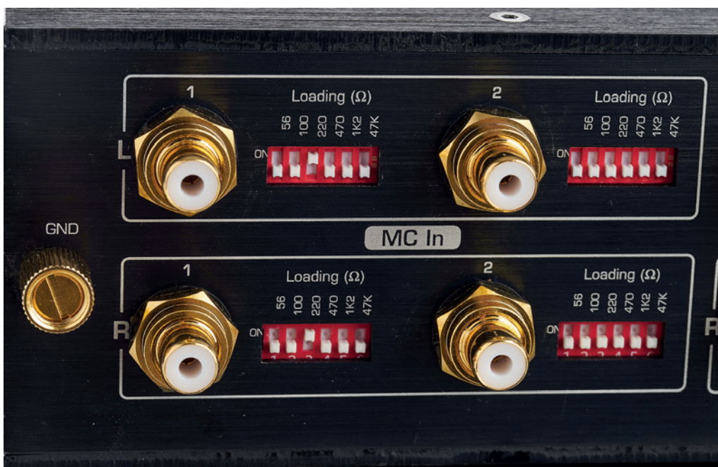
For each of the two MC inputs, six load impedances or combinations thereof are adjustable
