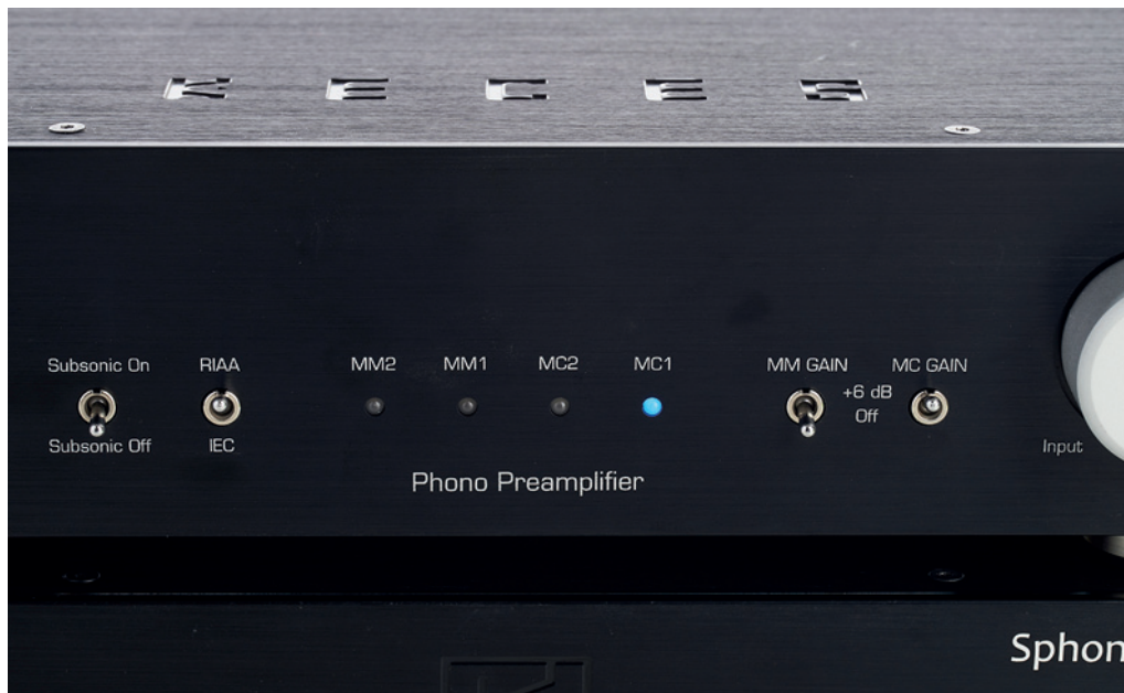
The front panel and its controls: The rotary switch for selecting the inputs, next to it the gain switches for MM and MC cartridges, followed by the switch for selecting the type of equalization, and the subsonic filter
