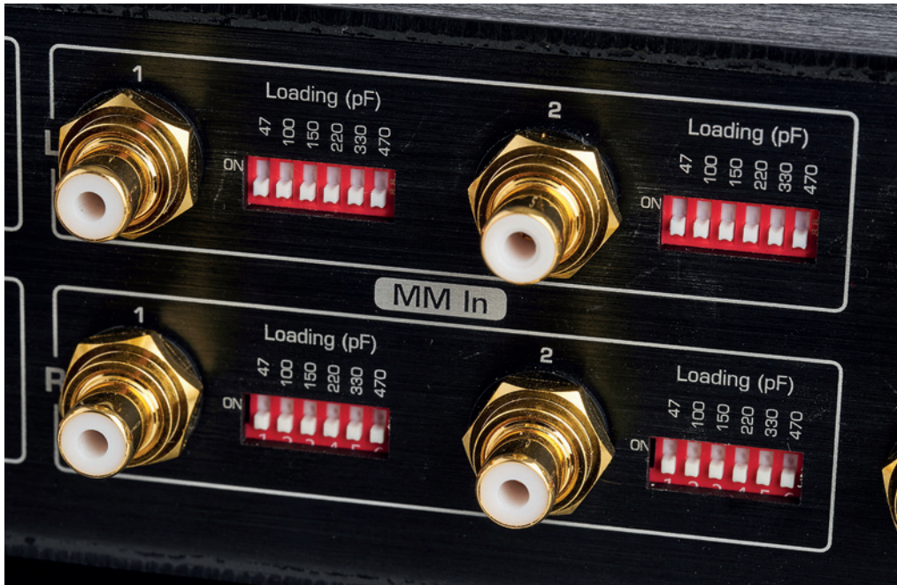
The two MM inputs can be terminated with six load capacities each
